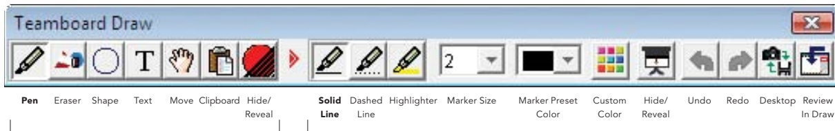
TeamBoard Annotation Bar: Interactive Mode Only – (Pen Tool selected with Solid Line option)
