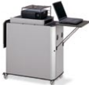
S2PM 202 Mobile Projector Center Design features include lockable cabinet lids that fold out at each end. Release the foot-lock and a gas-cylinder scissor-lift gently raises the projector. Lightly "push-down" to retract the mechanism. A low center of gravity and 3" locking casters ensure safe and easy mobility. Lid: Etex; Cabinet: Wood Veneer or Etex. 32"w x 34"h x 18"d
